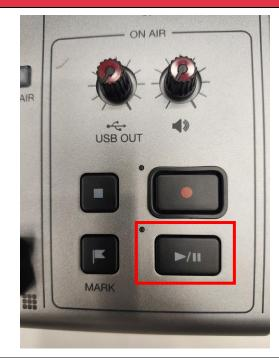
To Stop a recording and make a new file, press the square stop button 3 Note: Only do this if you want to END making an audio file
